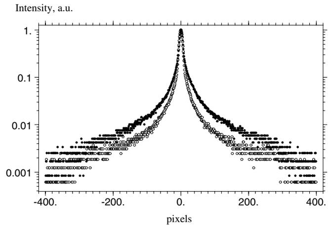
**Figure 4.** Intensity distribution perpendicular to the diffraction plane for the 25  $\mu\text{m}$  thick SOI layer (solid circles); experimentally measured point spread function is shown for comparison (empty circles).
