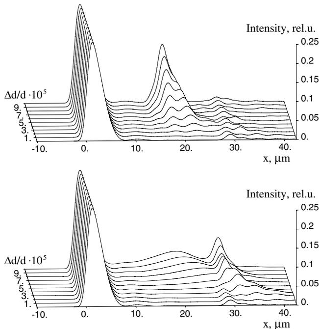
**Figure 3.** Theoretical simulations of the diffraction pattern from the 15  $\mu\text{m}$  thick Si layer (220 reflection, 9.5 keV) having the strain of a different origin. Top: a step-like interface between two layers of different lattice constants, located at a depth of 8  $\mu\text{m}$  below the surface. Bottom: linear  $\Delta d/d$  profile representing elastic bending of the layer.
