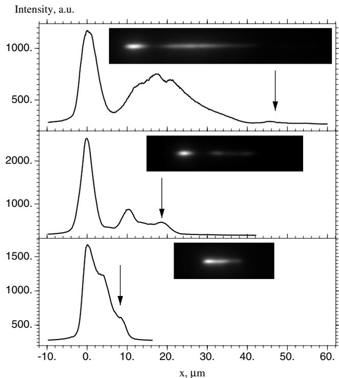
**Figure 2.** CCD diffraction images and their cross-sections by the diffraction plane recorded from the SOI layers of different thicknesses:  $25 \mu\text{m}$ , (2 2 0) reflection, upper panel;  $10 \mu\text{m}$ , (1 1 1), centre and  $4.5 \mu\text{m}$ , (2 2 0), bottom. The arrows show the position of the back surface.
