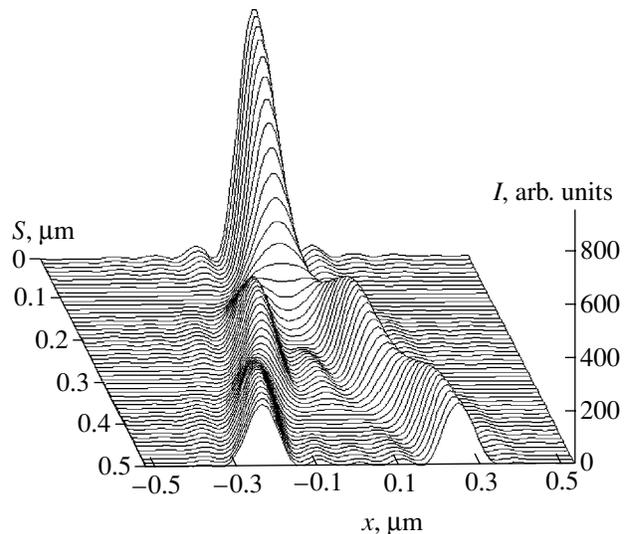
**Fig. 5.** Distribution of the relative intensity across the optical axis at different transverse displacements  $S$  between the two zone plates in the case of their close alignment ( $L = 0$ ).
