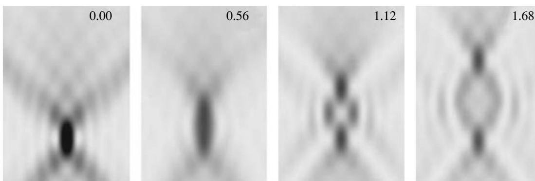
**Fig. 2.** 2D  $(x, z)$  distributions of the relative intensity near the focus at different longitudinal displacements of the second zone plate with respect to the first zone plate. The intensity is shown by linear scale of blackening from 0 (white) to 550 (black). The sizes of the model region in the horizontal and vertical directions are  $1.08 \mu\text{m}$  and  $4 \text{ mm}$ , respectively. The longitudinal displacement  $L$  (in mm) is indicated in the images.
