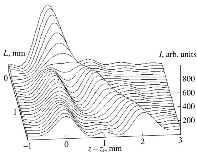
**Fig. 3.** Distribution of the relative intensity along the optical axis at different distances  $L$  between the two zone plates.
