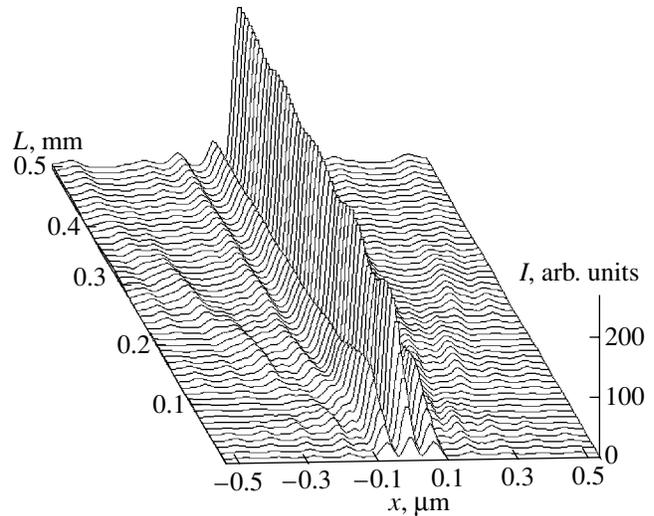
**Fig. 4.** Distribution of the relative intensity in the double focus (at the distance  $z_f(1, 1)$ ) at different distances between the two identical zone plates with a phase shift of  $\pi$  in each plate.
