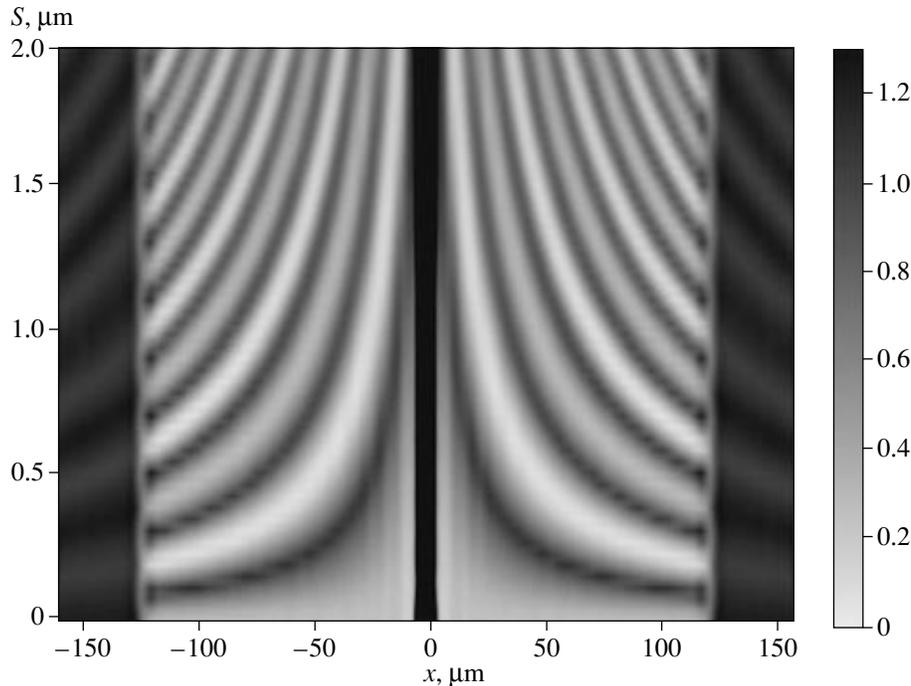
**Fig. 6.** Interference (moiré) pattern in the aperture region at a transverse displacement  $S$  between the two zone plates in the case of their close alignment ( $L = 0$ ).
