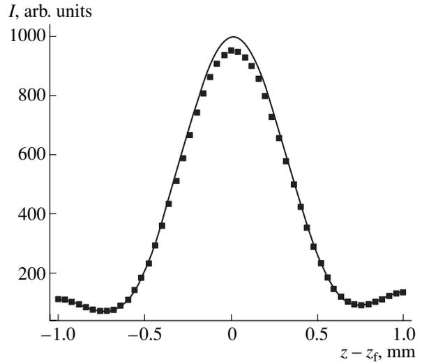
**Fig. 1.** Dependence of the relative intensity along the optical axis near the focus. Comparison of (squares) the fast Fourier transform data with (solid line) the results of the exact calculation.
